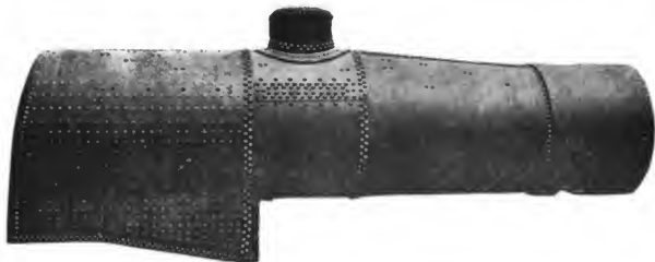
Fig. 145. Extended Wagon Top Boiler with Narrow Firebox.
